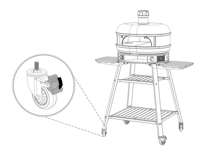
Always disconnect the oven from the gas supply before moving the oven.
